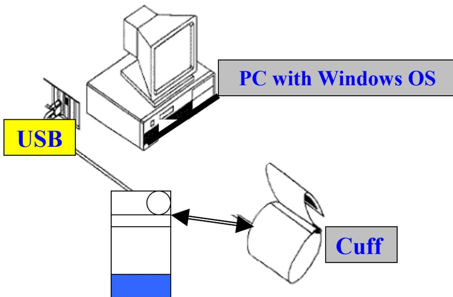
**Equipment Layout – Shown a DP-5200A/Pathway monitor (battery operation) connected with a cuff assembly and to a PC's USB communication port**
